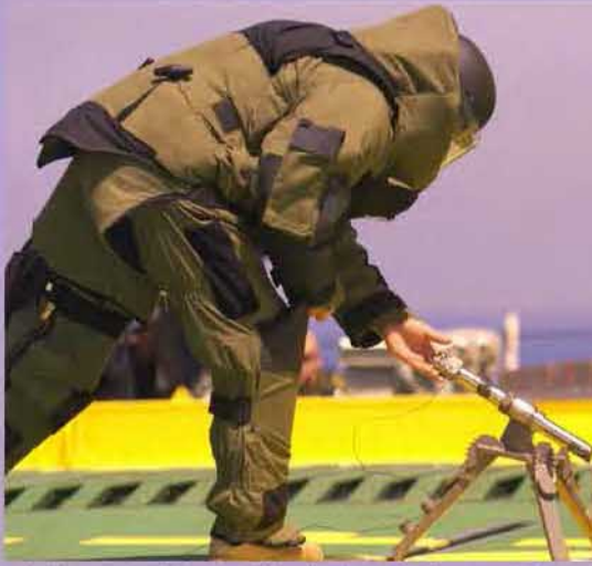
A clearance diver and Explosives Ordnance Disposal (EOD) expert aims a 20mm Neutrex Cannon to render safe a simulated improvised explosive device, during training aboard HMCS REGINA in the Strait of Hormuz.
